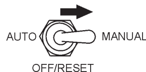
Figure 40. MPEC Control Switch (Manual Position)
