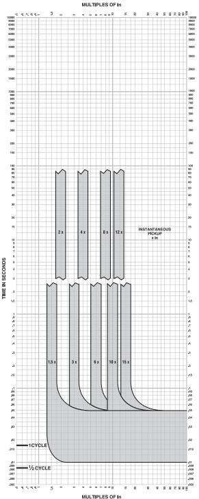
MICROLOGIC™ ELECTRONIC TRIP UNITS Micrologic™ 3.2/3.25/5.2A or E/6.2A or E Instantaneous Trip Curve 60A, 100A, 150A H-Frame
