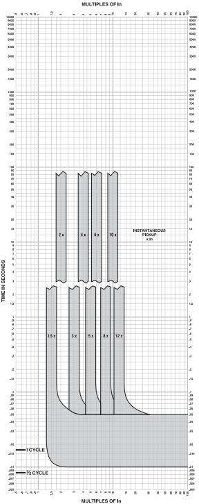
MICROLOGIC™ ELECTRONIC TRIP UNITS Micrologic™ 3.3, 3.3-W, 3.3S, 3.3S-W, 5.3A, 5.3A-W, 5.3E, 5.3E-W, 6.3A, 6.3A-W, 6.3E, and 6.3E-W Instantaneous Trip Curve 400A L-Frame
