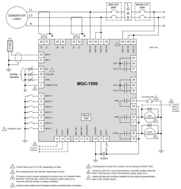
Figure 52. Single-Phase A-C Connections for Typical Applications
