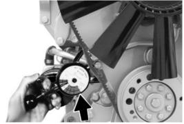
Checking Belt Tension with Tension Gauge
