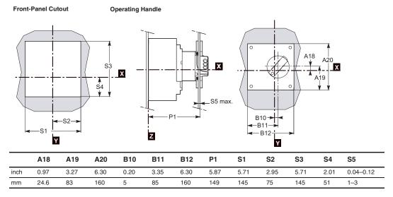
Figure 50: PowerPact L-Frame Circuit Breaker Extended Rotary Handle Mounting
