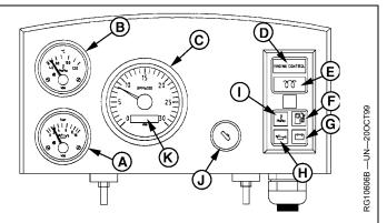
A—Oil Pressure Gauge B—Coolant Temperature
