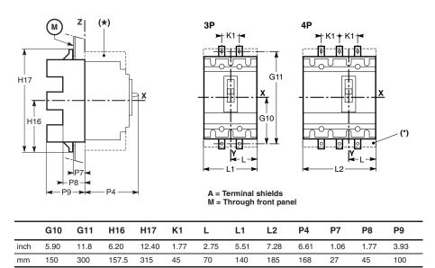
Figure 41: PowerPact L-Frame Drawout Circuit Breaker (on Cradle)
