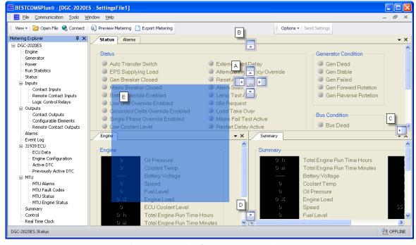
Figure 26. Metering Screen Docking Options
