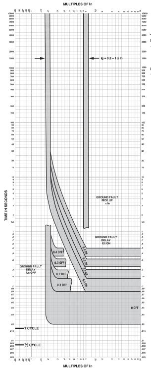
MICROLOGIC™ ELECTRONIC TRIP UNITS Micrologic™ 6.2A or E Ground Fault Trip Curve 100A, 150A H-Frame
