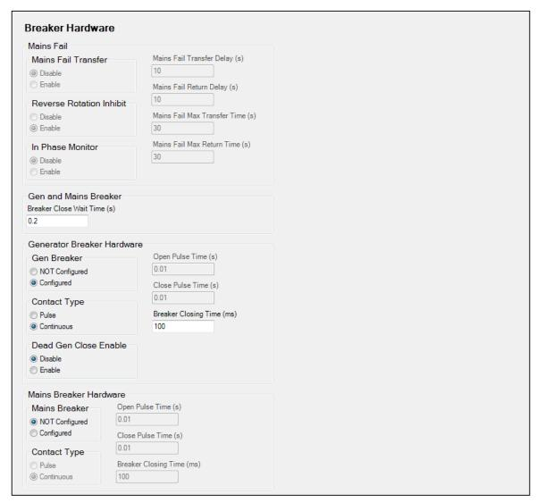
Figure 18. Settings Explorer, Breaker Management, Breaker Hardware Screen
