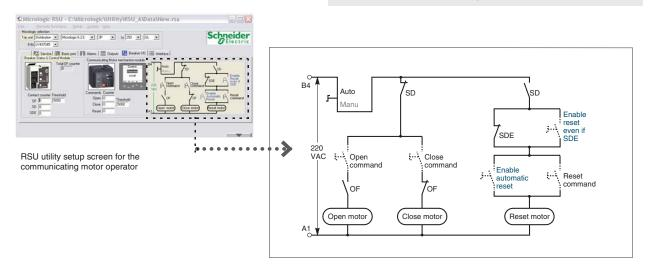
Single-line diagram of communicating motor operator
