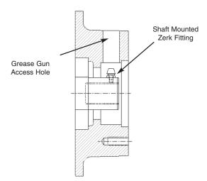
Figure 3--Drive End Bearing Bracket
