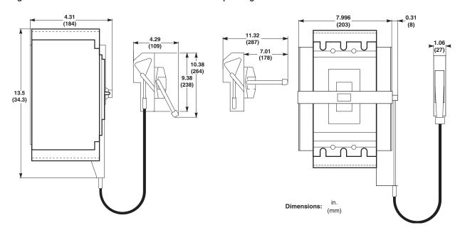
Figure 48: PowerPact L-Frame Circuit Breaker Rotary-Operating Handles
