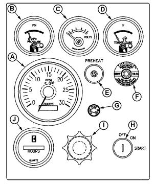
Instrument Panel and Gauges (Later Engines)
