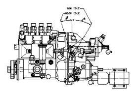
Figure 12-3: Standard Mechanical Governor for Diesel Engines
