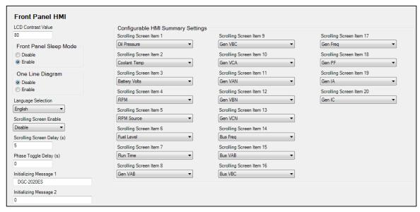
Figure 7. Settings Explorer, General Settings, Front Panel HMI Screen
