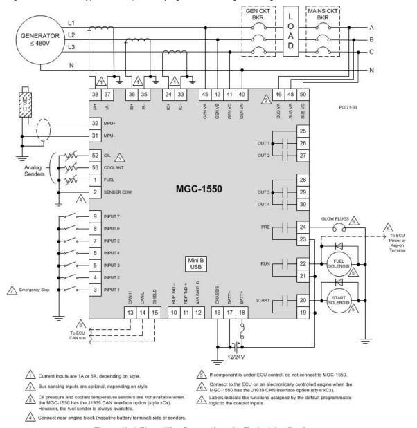
Figure 49. 3-Phase Wye Connections for Typical Applications
