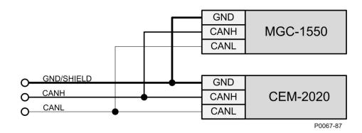
Figure 55. MGC-1550 and CEM-2020 CAN Connections
