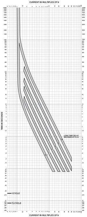
MICROLOGIC™ ELECTRONIC TRIP UNITS Micrologic™ 5.2A, 5.2A-W, 5.2E, 5.2E-W, 6.2A, 6.2A-W, 6.2E, and 6.2E-W Long Time Trip Curve 250A J-Frame
