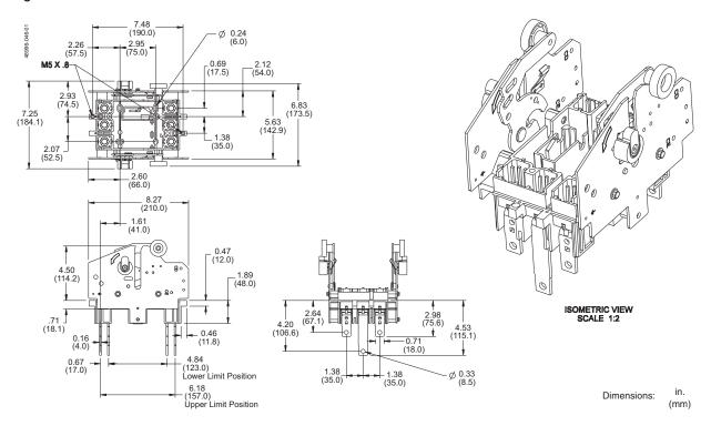
Figure 28: 15–250 A PowerPact H- and J-Frame Drawout Three-Pole Circuit Breaker
