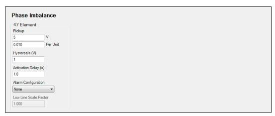
Figure 23. Settings Explorer, Generator Protection, Voltage, Phase Imbalance (47) Screen
