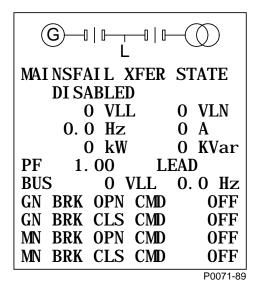
Figure 5. One-Line Diagram Menu Options (Available when One-Line Diagram is Enabled)
