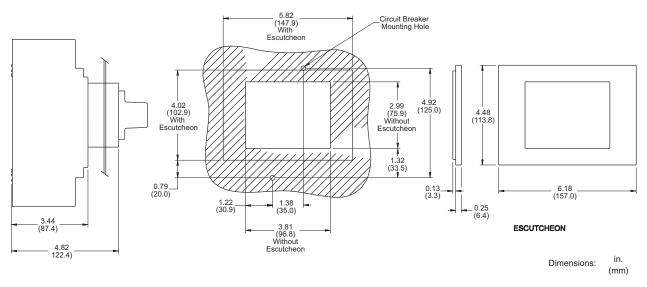
Figure 34: PowerPact H- and J-Frame Circuit Breaker Door Mounted Rotary Handle Cutout
