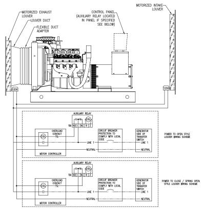
Figure 8-8: Suggested motorized louver wiring
