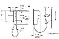
Refer to NEC Article 430-10 for minimum dimension X from circuit breaker top mounting hole to wall or barrier to ensure adequate wire bending space.
