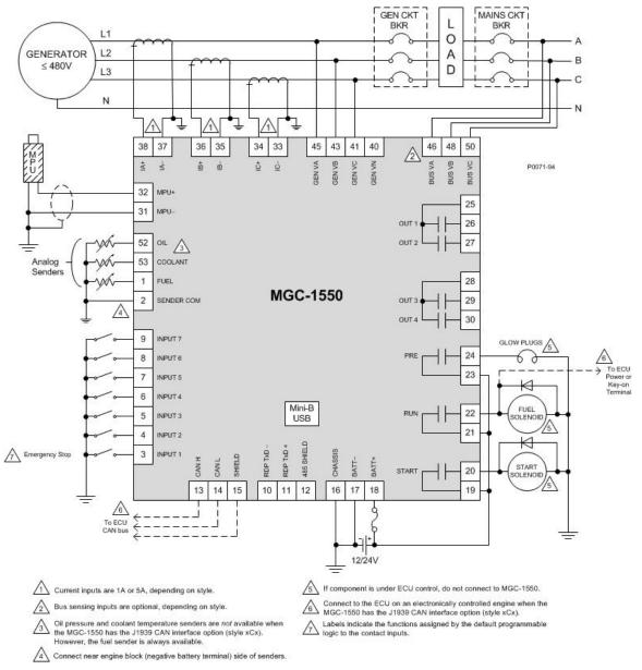
Figure 50. 3-Phase Delta Connections for Typical Applications
