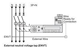
This connection is required for accurate power measurements on three-pole circuit breakers equipped with Micrologic 5/6 E trip units in installations with a distributed neutral. It can be used to measure phase-neutral voltages and calculate power using the 3 wattmeter method.
