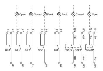
**NOTE:** Schematic of the communicating motor operator .
