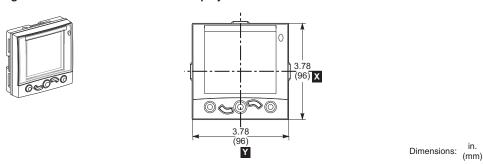
Figure 65: FDM121 Switchboard Display Mounting Through Panel
