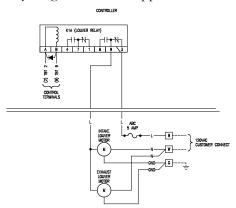
Figure 8-9: Optional motorized louver wiring
