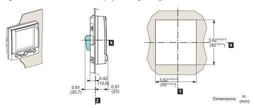
Figure 66: FDM121 Switchboard Display Mounting On Panel
