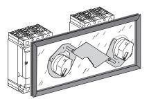
Interlocking with Rotary Handles (S29369)
