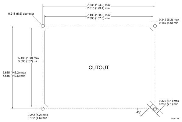
Figure 46. Panel Cutting and Drilling Dimensions
