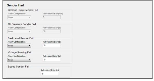
Figure 43. Settings Explorer, Alarm Configuration, Sender Fail Screen
