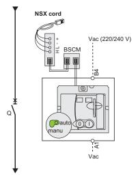
$\label{NOTE: NOTE: Schematic of the communicating motor operator} \ .$
