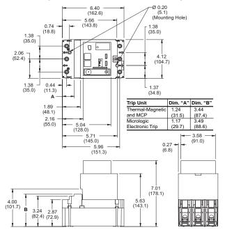
Figure 19: Rotary Handle Detail (PowerPact H-Frame Circuit Breaker)
