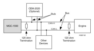
Figure 95. CAN Interface with MGC-1550 providing One End of the Bus
