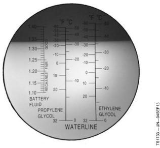
Image with a Drop of 50/50 Coolant Placed on the Refractometer Window
