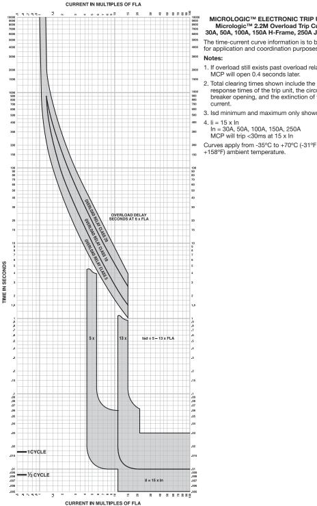
MICROLOGIC™ ELECTRONIC TRIP UNITS Micrologic™ 2.2M Overload Trip Curve 30A, 50A, 100A, 150A H-Frame, 250A J-Frame
