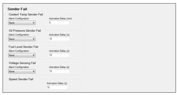
Figure 11. Settings Explorer, Alarm Configuration, Sender Fail Screen
