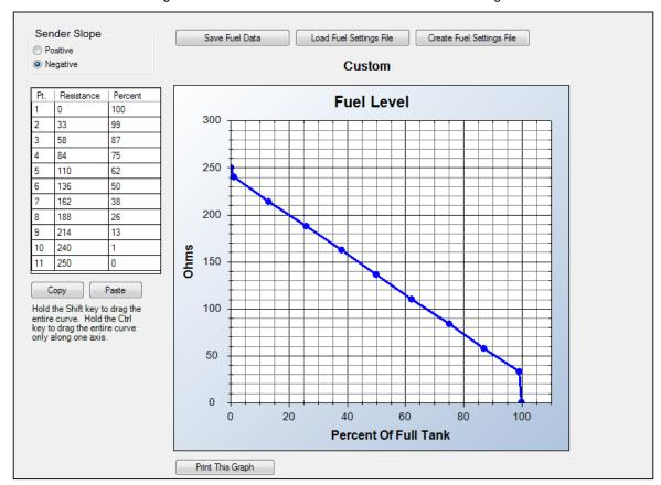
Figure 8. Settings Explorer, Programmable Senders, Fuel Level Screen
