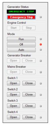
Figure 38. Metering Explorer, Control Screen
