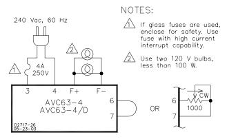
Figure 9. Operational Test Diagram
