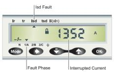
On a fault trip, the type of fault  $(I_r, I_{sd}, I_i, I_g)$ , the phase concerned and the interrupted current are displayed. An external power supply is required.
