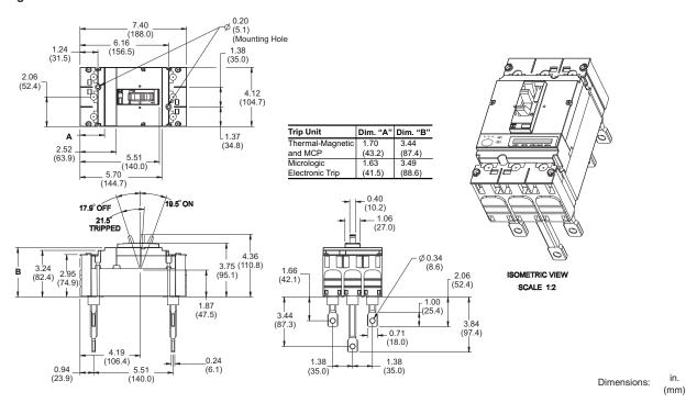
Figure 18: Motor Operator Detail (PowerPact H-Frame Circuit Breaker)
