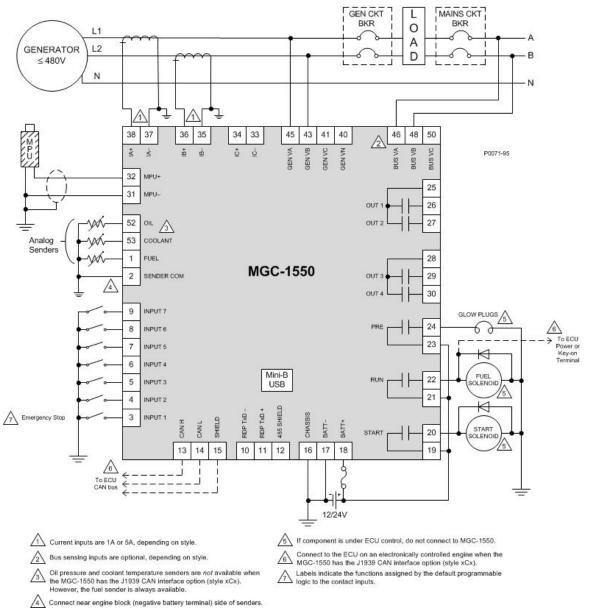
Figure 51. Single-Phase A-B Connections for Typical Applications
