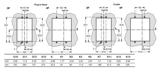
Figure 43: PowerPact L-Frame Circuit Breaker Mounting on Rails (Plug-In Base or Cradle)
