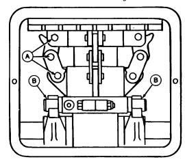
Lubrication Internal Parts of PTO Clutch
