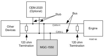
Figure 54. CAN Interface with Other Devices
