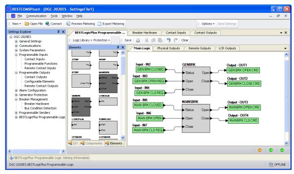
Figure 19. Settings Explorer, BESTlogic Plus Programmable Logic Screen
