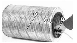
Inspecting Primary Air Filter Element
