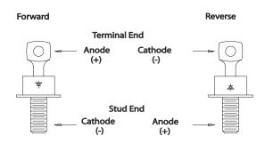
FIGURE 4: DIODE POLARITY
