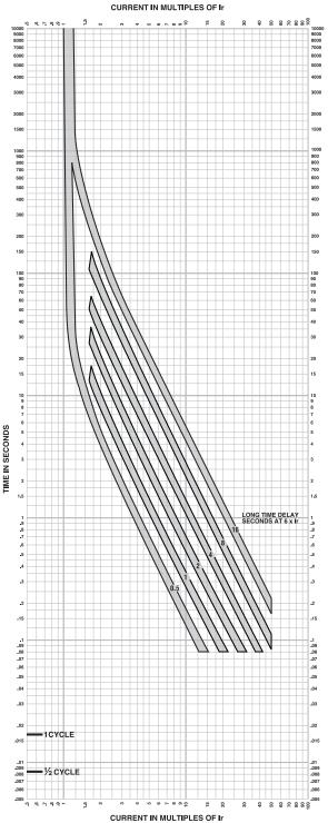
MICROLOGIC™ ELECTRONIC TRIP UNITS Micrologic™ 5.3A, 5.3A-W, 5.3E, 5.3E-W, 6.3A, 6.3A-W, 6.3E, and 6.3E-W Long Time Trip Curve 600A L-Frame
