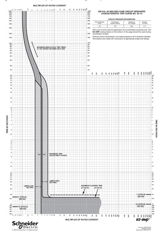
Figure 80: J-Frame 150 A (JG) 500 Vdc Thermal-Magnetic Trip
