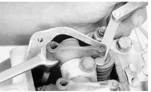
Checking Valve Clearance
