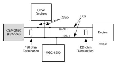
Figure 94. CAN Interface with CEM-2020 providing One End of the Bus
