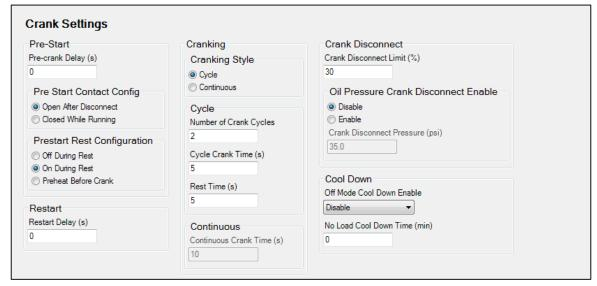
Figure 84. Settings Explorer, System Parameters, Crank Settings Screen
