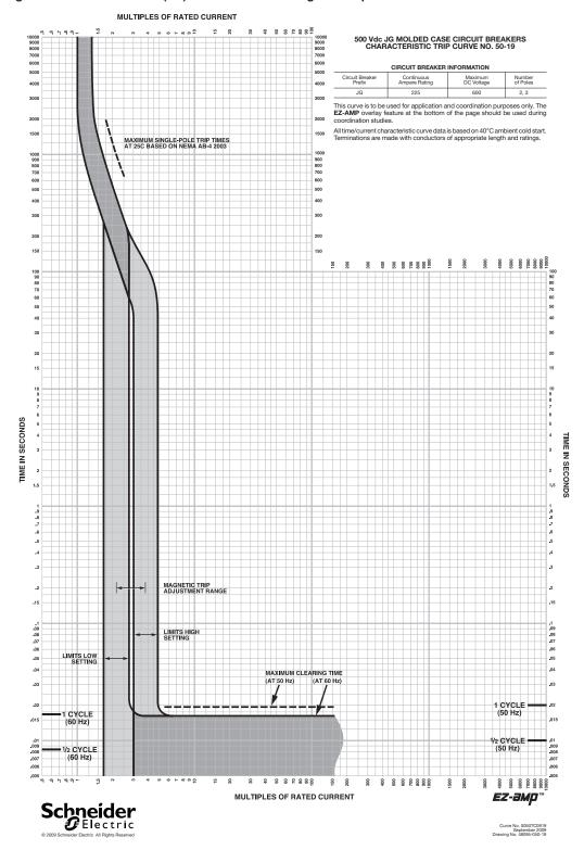
Figure 84: J-Frame 250 A (JG) 500 Vdc Thermal-Magnetic Trip
