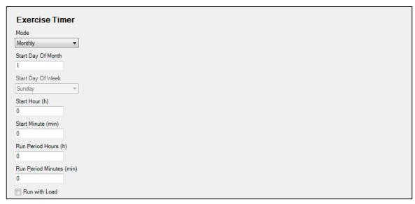
Figure 86. Settings Explorer, System Parameters, Exercise Timer Screen
