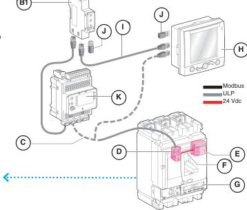
Communication Components and Connections, IFE Ethernet
