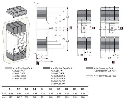
Figure 37: PowerPact L-Frame Circuit Breaker Mounting
