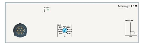
Micrologic 1.3 M trip units provide instantaneous protection only, using electronic technology. They are dedicated to 600 A three-pole (3P 3D) circuit breakers or four-pole circuit breakers with detection on three poles (4P, 3D). They are especially used in three-pole versions for motor protection.
