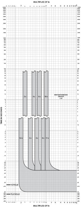
MICROLOGIC™ ELECTRONIC TRIP UNITS Micrologic™ 3.3, 3.3-W, 3.3S, 3.3S-W, 5.3A, 5.3A-W, 5.3E, 5.3E-W, 6.3A, 6.3A-W, 6.3E, and 6.3E-W Instantaneous Trip Curve 600A L-Frame
