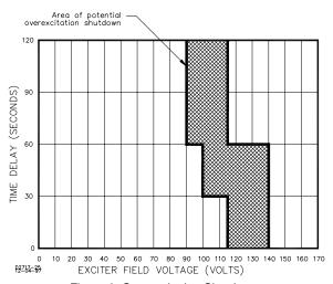
Figure 6. Overexcitation Shutdown Time Delay Characteristic
