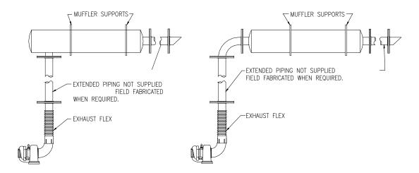
Figure 6-1: Typical side inlet exhaust
