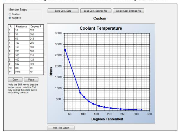
Figure 10. Settings Explorer, Programmable Senders, Coolant Temperature Screen
