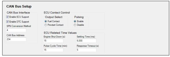
Figure 75. Settings Explorer, Communications, CAN Bus, CAN Bus Setup
