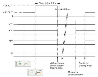
I: Charge Current SDT: Thermal Fault Signal
