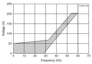
Figure 4. Frequency Compensation Characteristic - 60 Hz
