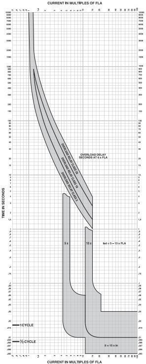
MICROLOGIC™ ELECTRONIC TRIP UNITS Micrologic™ 2.2M Overload Trip Curve 30A, 50A, 100A, 150A H-Frame, 250A J-Frame
