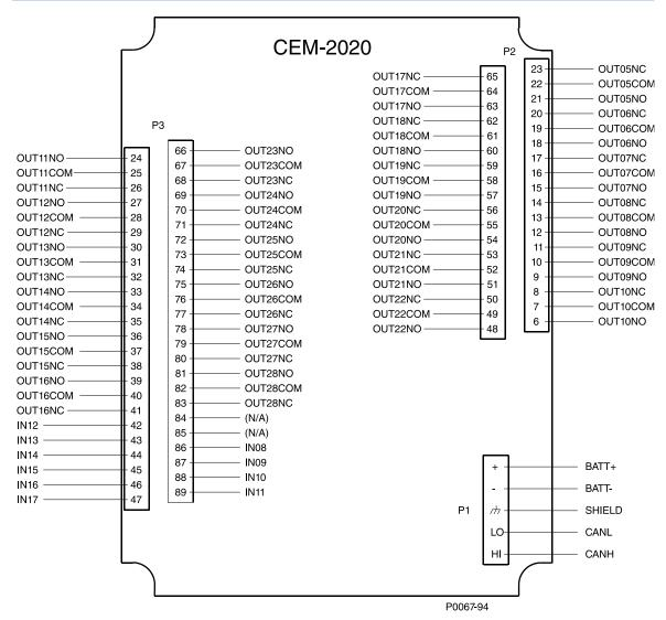
Figure 93. CEM-2020 Contact Input and Contact Output Terminals
