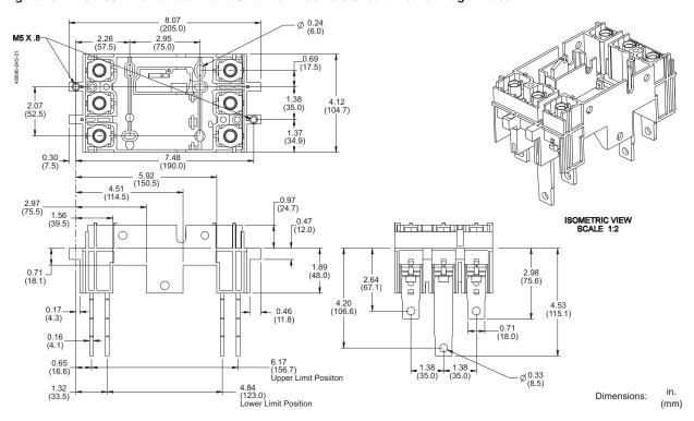
15-250 A PowerPact H- and J-Frame Plug-In Three-Pole Circuit Breaker
