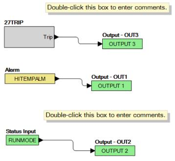
Figure 74. Example 3 – Multiple Logic Connections
