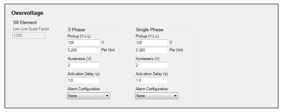
Figure 22. Settings Explorer, Generator Protection, Voltage, Overvoltage (59) Screen
