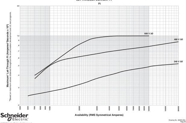
Figure 96: J-Frame UL Listed Current -Limiting Circuit Breaker
