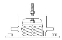
Figure 4-2: Spring mount vibration isolator
