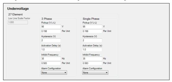
Figure 21. Settings Explorer, Generator Protection, Voltage, Undervoltage (27) Screen
