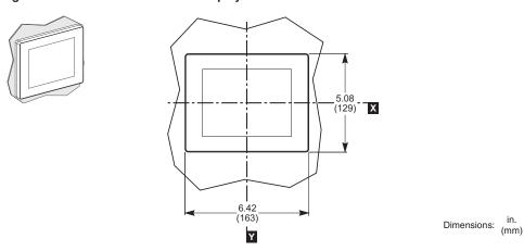
Figure 68: FDM128 Switchboard Display Mounting on Panel
