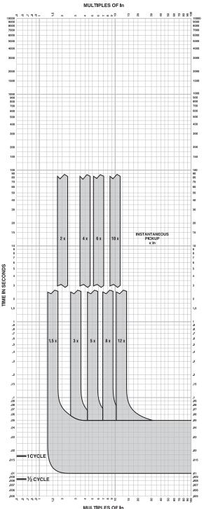
MICROLOGIC™ ELECTRONIC TRIP UNITS Micrologic™ 3.2, 3.2-W, 3.2S, 3.2S-W, 5.2A, 5.2A-W, 5.2E, 5.2E-W, 6.2A, 6.2A-W, 6.2E, and 6.2E-W Instantaneous Trip Curve 250A J-Frame
