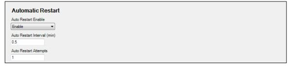
Figure 85. Settings Explorer, System Parameters, Automatic Restart Screen
