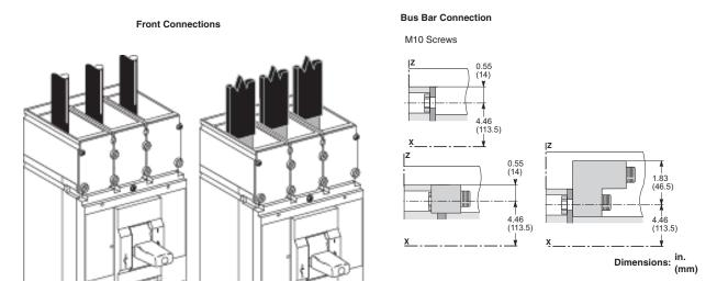
Figure 57: PowerPact L-Frame Circuit Breaker Rear Connections
