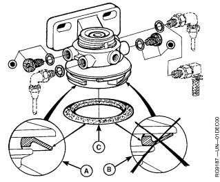
Fuel Filter Dust Seal Installation
