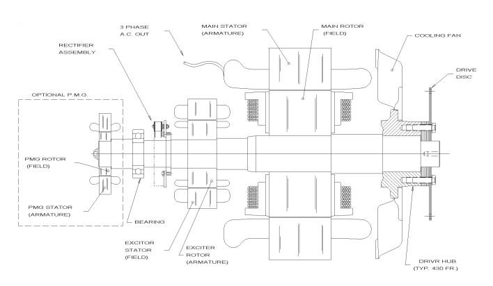
FIGURE 2 -- Typical MagnaPLUS® Layout Diagram
