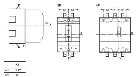
Figure 59: PowerPact L-Frame Circuit Breaker Rear Connections Fitted at Lower Limit
