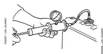
Pressure Testing Cooling System
