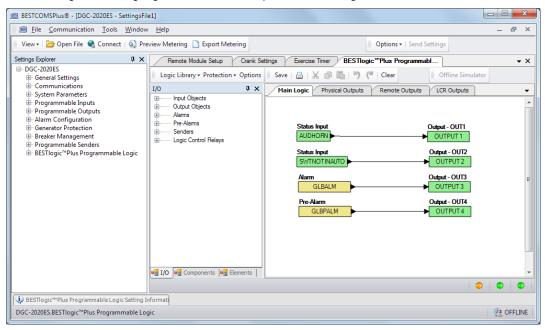
Figure 68. Settings Explorer, BESTlogic Plus Programmable Logic Screen
