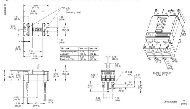
Figure 23: Motor Operator Detail (PowerPact J-Frame Circuit Breaker)
