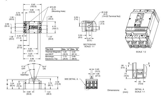
Figure 16: 15-150 A Lug-Lug PowerPact H-Frame Three-Pole Circuit Breaker
