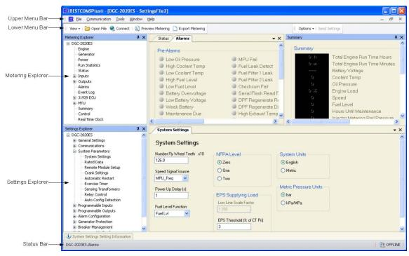
Figure 56. Typical User Interface Components
