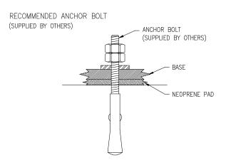
Figure 4-3: Recommended anchor bolt
