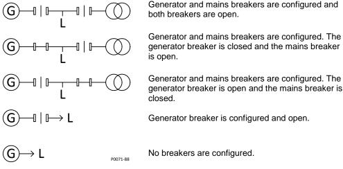
Figure 6. One-Line Diagram: Breaker Hardware Status Indication
