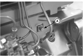
Engine Block Drain Valve
