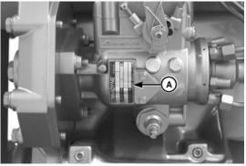
Injection Pump Serial Number Plate
