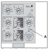
Figure 5: Micrologic 6.0A Trip Unit
