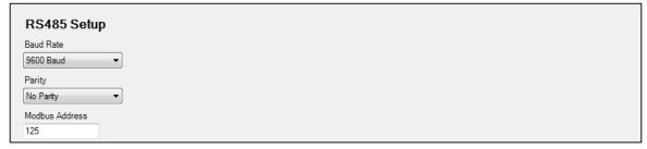
Figure 77. Settings Explorer, Communications, RS485 Setup
