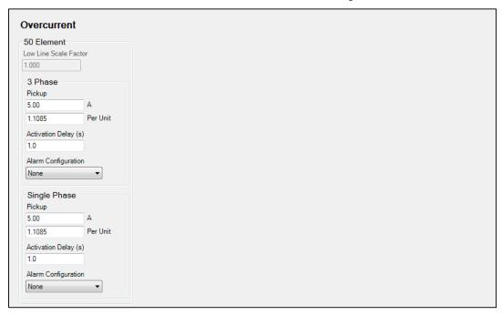
Figure 25. Settings Explorer, Generator Protection, Current, Overcurrent
