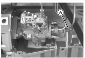
Fuel Supply Line Connector at Injection Pump
