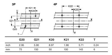
**PowerPact L-Frame Circuit Breaker Front-Panel Cutouts**
