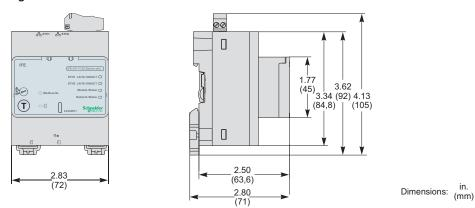
Figure 62: I/O (Input/Output) Application Module
