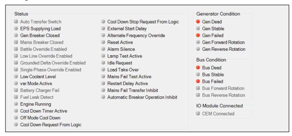
Figure 31. Metering Explorer, Status Screen
