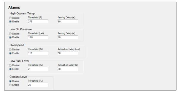
Figure 40. Settings Explorer, Alarm Configuration, Alarms Screen
