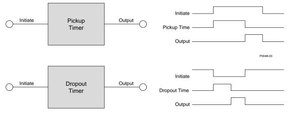
Figure 69. Pickup and Dropout Timer Logic Blocks
