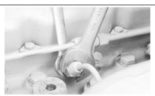
Bleeding Fuel System at Injection Nozzle
