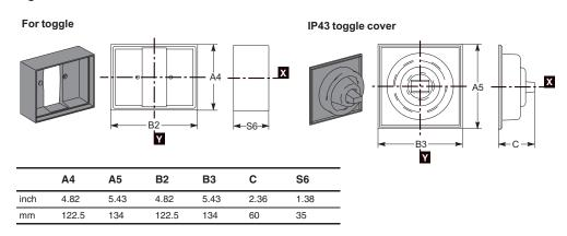
Figure 52: PowerPact L-Frame Circuit Breaker Front-Panel Escutcheons
