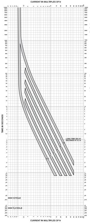
MICROLOGIC™ ELECTRONIC TRIP UNITS Micrologic™ 5.3A, 5.3A-W, 5.3E, 5.3E-W, 6.3A, 6.3A-W, 6.3E, and 6.3E-W Long Time Trip Curve 400A L-Frame
