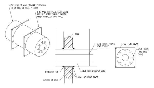
Figure 6-3: Wall thimble installation
