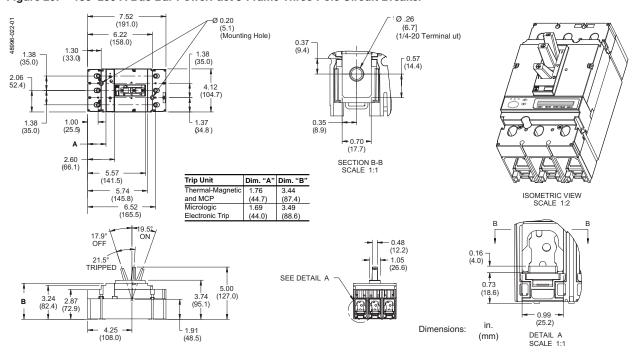
Figure 21: 150-250 A Lug-Lug PowerPact J-Frame Three-Pole Circuit Breaker
