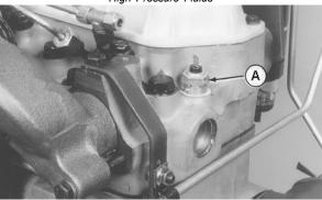
Coolant Temperature Sending Unit Fitting
