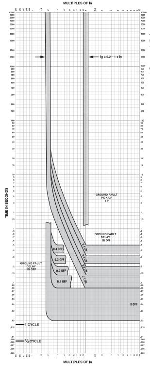
MICROLOGIC™ ELECTRONIC TRIP UNITS Micrologic™ 6.3A, 6.3A-W, 6.3E, and 6.3E-W Ground Fault Trip Curve 400A, 600A L-Frame
