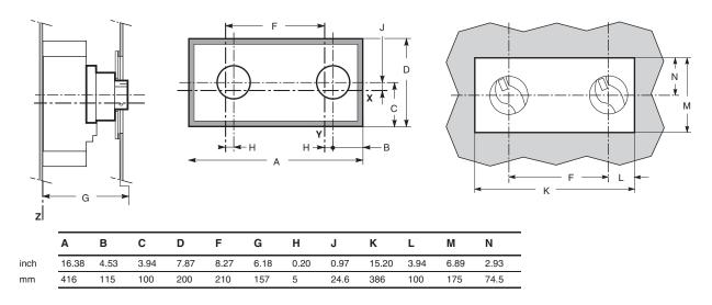
Figure 54: PowerPact L-Frame Circuit Breaker Interlocking Systems with Toggle Handles
