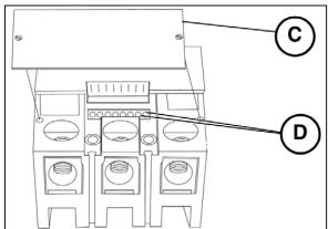
Figure 3: Lug cover for access to terminals 7 and 8
