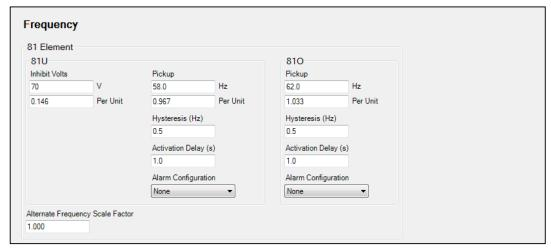
Figure 24. Settings Explorer, Generator Protection, Frequency, Frequency (81) Screen
