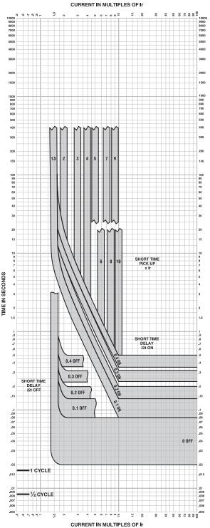
MICROLOGIC™ ELECTRONIC TRIP UNITS Micrologic<sup>™</sup> 5.3A, 5.3A-W, 5.3E, 5.3E-W, 6.3A, 6.3A-W, 6.3E, and 6.3E-W Short Time Trip Curve 400A L-Frame
