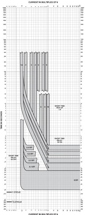
MICROLOGIC™ ELECTRONIC TRIP UNITS Micrologic™ 5.3A, 5.3A-W, 5.3E, 5.3E-W, 6.3A, 6.3A-W, 6.3E, and 6.3E-W Short Time Trip Curve 600A L-Frame
