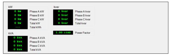
Figure 29. Metering Explorer, Power Screen
