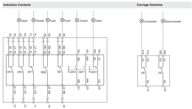
$The \ diagram \ is \ shown \ with \ circuits \ de-energized, \ relays \ in \ normal \ position, \ and \ all \ devices \ open, \ connected, \ and \ charged.$
