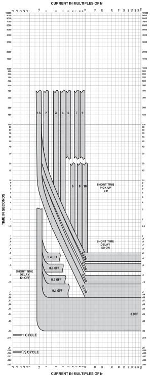
MICROLOGIC™ ELECTRONIC TRIP UNITS Micrologic™ 5.2A, 5.2A-W, 5.2E, 5.2E-W, 6.2A, 6.2A-W, 6.2E, and 6.2E-W Short Time Trip Curve 250A J-Frame
