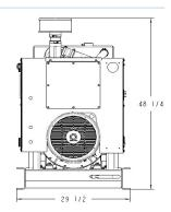
Drawing above for illustration purposes only, based on standard open power 480 volt generator set. Lengths may vary with other voltages. Do not use for installation design. See website for unit specific template drawings.
