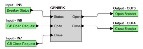
Figure 72. Example 1 - GENBRK Logic Block Connections
