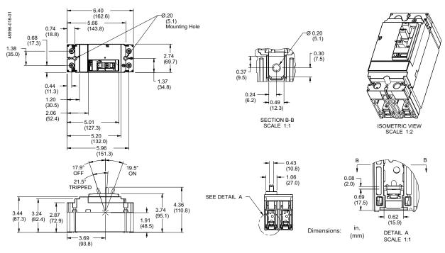
15-150 A Unit Mount PowerPact H-Frame Two-Pole HD/HG Thermal-Magnetic Only Circuit Breaker Figure 14:
